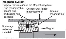
For this sensor principle it is not sufficient to simply mount the permanent magnet onto the piston. A magnetic system has to be constructed which conducts the magnetic flux of the permanent magnets directlt into the cylinder wall in order to achieve the strongest possible magnetization. For further details regarding the construction of magnetic systems, refer to the manual. A field trial is generally recommended before practical operation!
